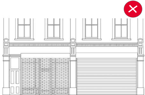
Picture 23. External Roller shutters are not appropriate.
